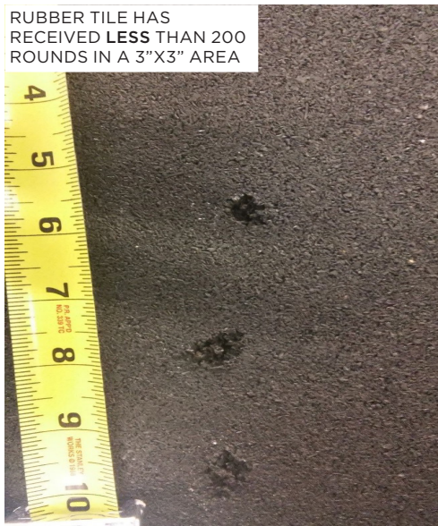
FIGURE 21. FRONT SIDE OF RUBBER PANEL DOES NOT NEED TO BE REPLACED
