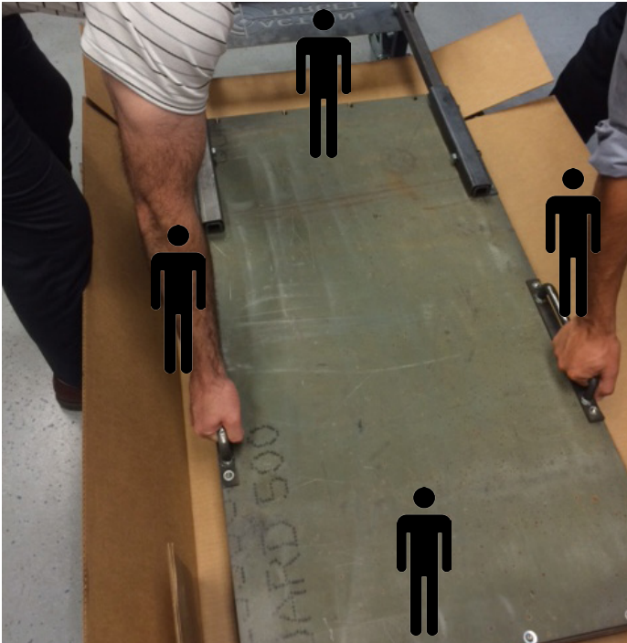
FIGURE 12. POSITIONS OF PERSONS LIFTING THE BULLET TRAP PLATE
