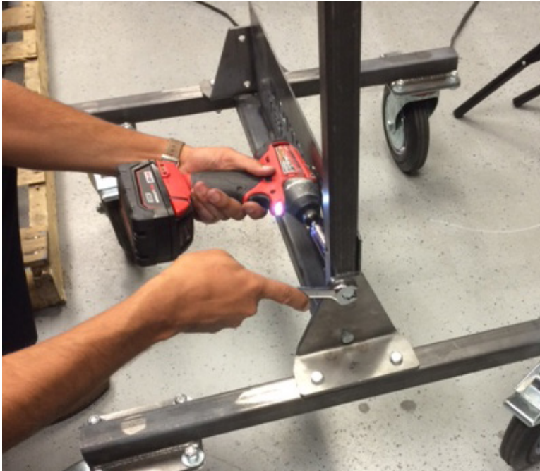
FIGURE 7. TIGHTENING FLAT WASHERS AND STOVERS ONTO CARRIAGE BOLTS
