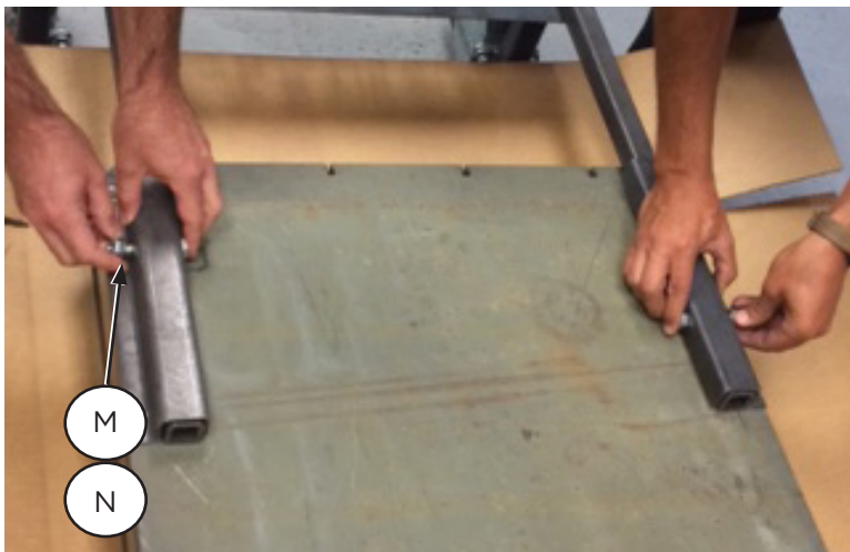
FIGURE 11. INSTALLING WASHERS AND NUTS TO HEX BOLTS
