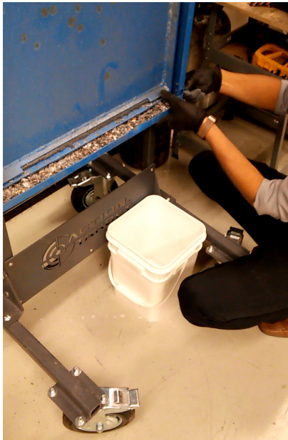
FIGURE 16. UNDO LATCH ON SIDE OF BULLET FRAGMENT TRAY
