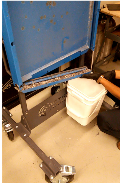
FIGURE 17. HOLD BUCKET BENEATH TRAY AS IT IS LOWERED
