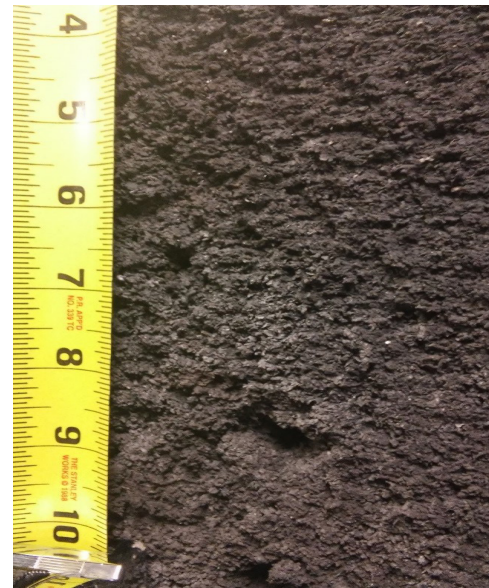
FIGURE 22. BACK SIDE OF RUBBER PANEL DOES NOT NEED TO BE REPLACED
